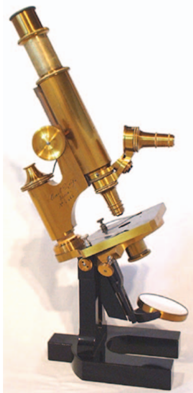
Figure 9 - Zeiss Microscope 1879, with Abbe's optics.
