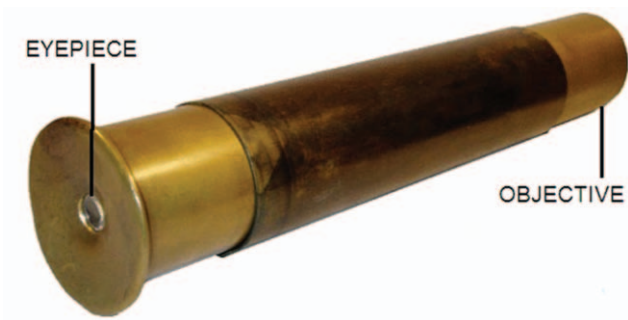
Figure 5 - The first microscope designed by Hans and Zacharias Janssen.
